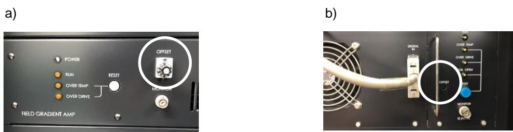
Fig. 5: The offset adjustment knob on a 10 A FG amplifier a), and the offset adjustment screw on a 30 A FG amplifier.
