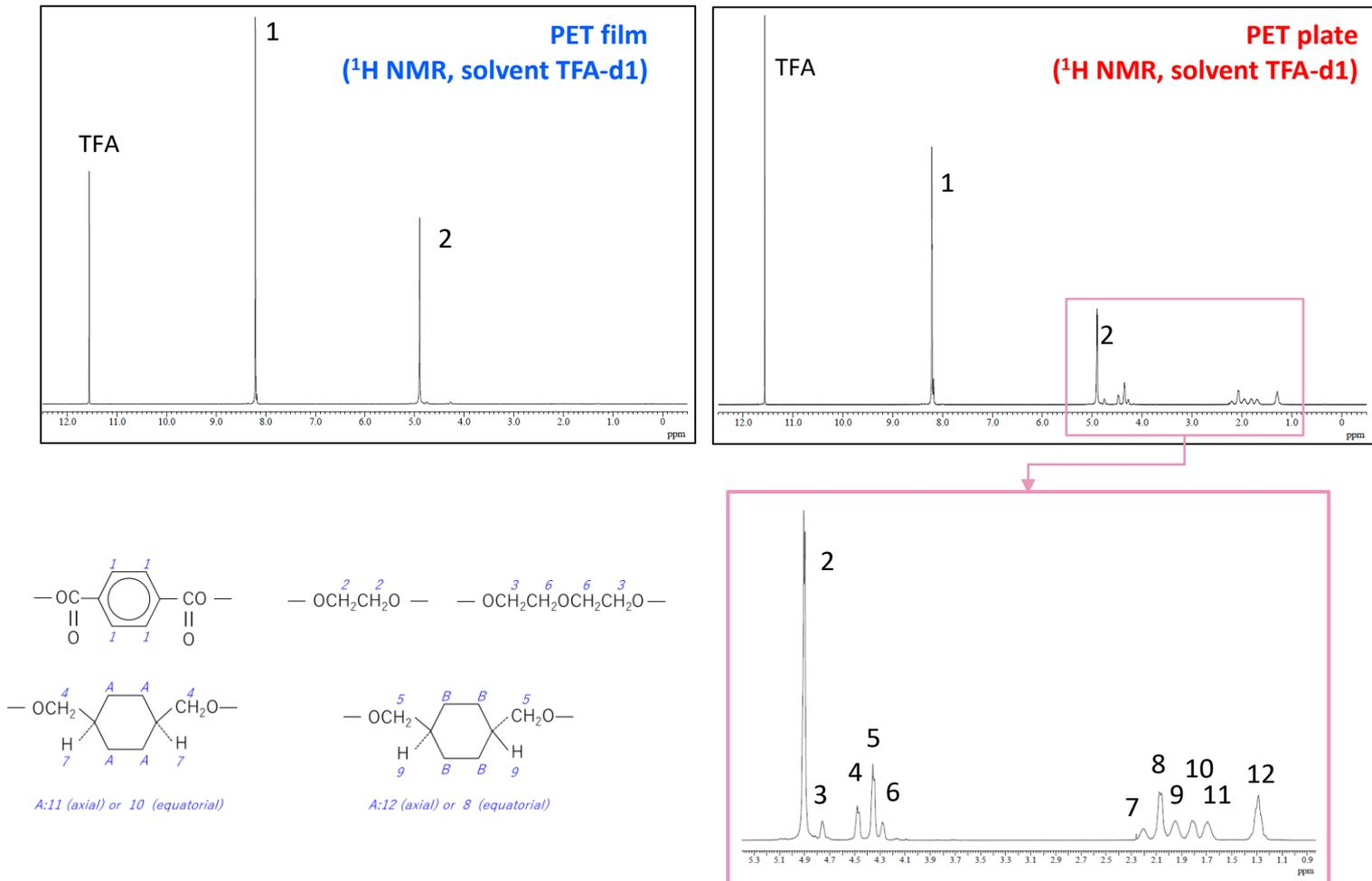
Figure 5 <sup>1</sup>H NMR spectra of PET film and PET plate
