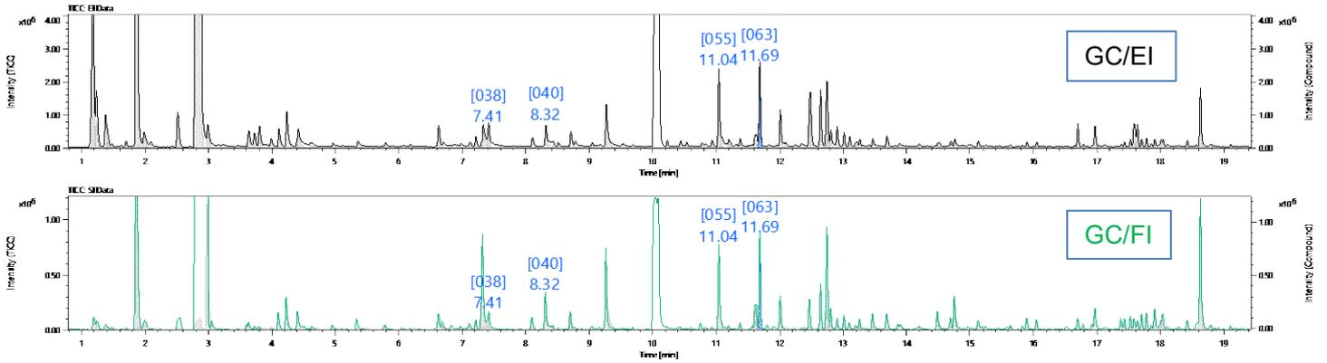
Figure 2: Py-GC-EI and FI TIC chromatograms for an Methyl methacrylate-methyl acrylate copolymer
