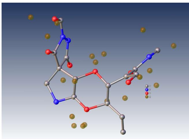
Initial structure model of Rhynchophylline, Electron diffraction structure analysis, XtaLAB Synergy-ED
