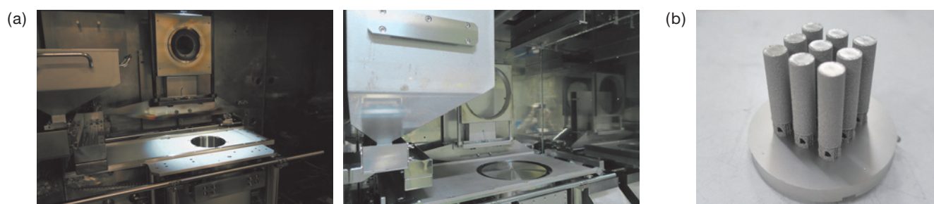
(a) Small-scale production option unit (left) and Standard unit (right), (b) Example of a build object (Ni718 alloy-based cylinder: 10 mm dia. x 50 mm).
