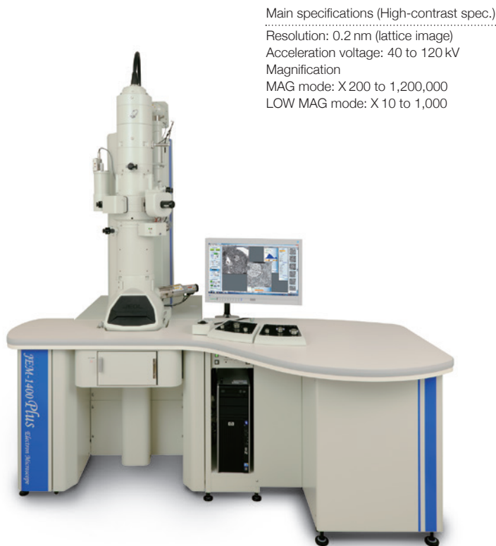
Fig. 1 JEM-1400Plus appearance and specifications
