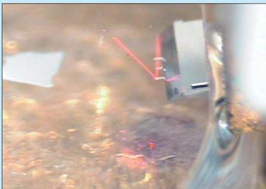
In-fluid observation when a cover glass is attached to the cantilever.
