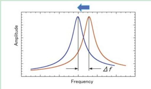
To set the frequency of the cantilever beam to the resonant frequency any time, PLL (Phase Locked Loop) is used. The FM detection method with PLL is a standard configuration of JEOL SPMs, which is an unprecedented feature of JEOL SPMs.
