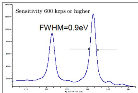
Ag3d photoelectron spectrum
