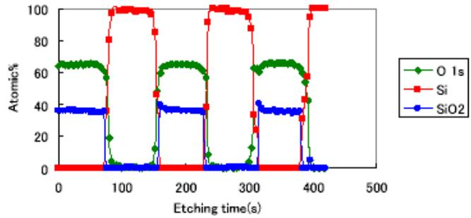
The figure below shows the depth profile of SiO<sub>2</sub> and Si obtained by the Depth Profile program. The data shows that each layer is 25 nm thick.
