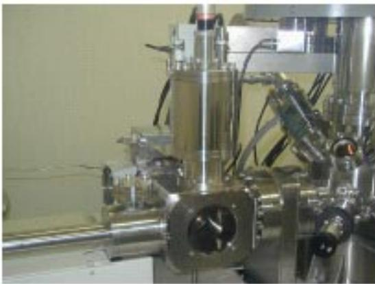
The high speed ion gun is specifically designed for XPS to etch samples at a low accelerating voltage from 150 V to 1500 V, minimizing the damage on the surface and interface. The etching rate is 3 to 120 nm/min ( $\text{SiO}_2$  conversion).
