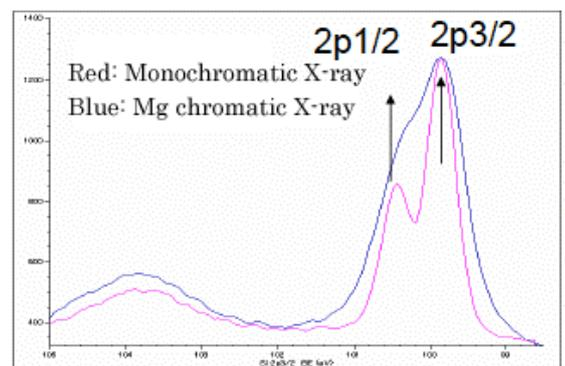
compares the Si2P spectra acquired with monochromatic and Mg chromatic X-rays.
