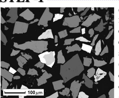
Samples taken from the minerals processing plant contain particle powders embedded in resin. In the back scattered electron (BSE) image (left), the contrast in the image corresponds to the composition of the minerals in the particles as captured in the scanning electron microscope (SEM).
