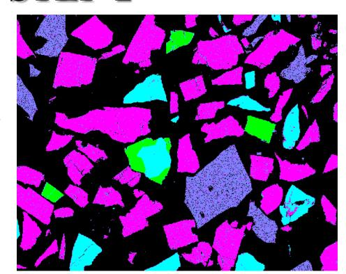
Grains and grain morphology are identified using the contrast in the BSE image. Morphological data like area, perimeter length, ECD and location of each grain is stored in a database for further processing. A grain can be classified from the BSE image or using the composition determined from an EDS measurement (Step 3).
