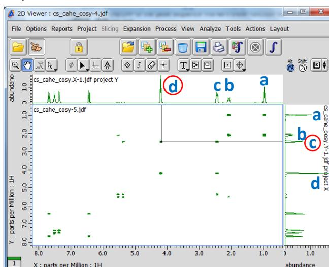
The peak sequence markers are shown as two perpendicular lines at **c** and **d** peaks
