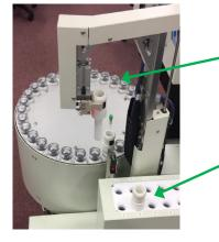
Room temperature slot (Returning sample from high temperature slot is put in here)
