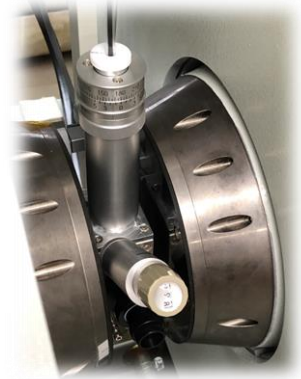
Fig. 1 ES-UCR3X (Angular rotation device).
