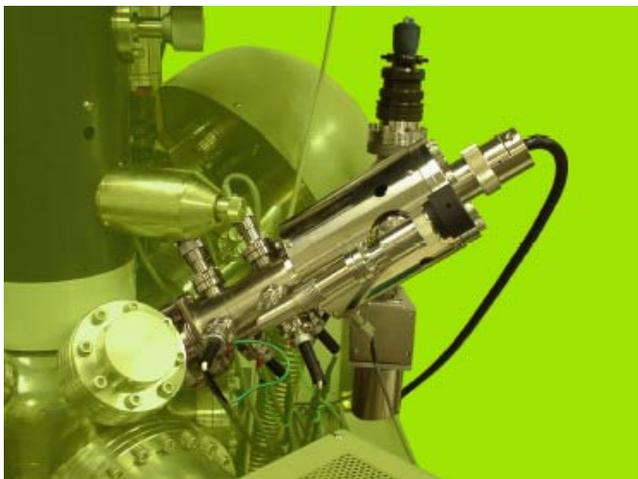
Figure: Floating micro ion etching device
