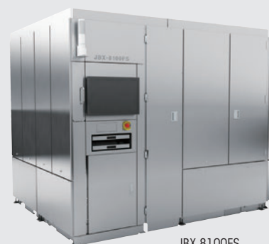
JBX-8100FS electron beam lithography system
