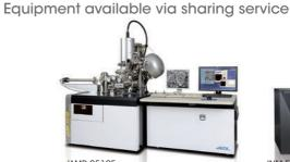
JAMP-9510F field emission Auger microprobe
