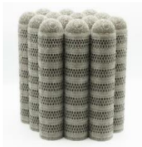
Material : Ti64 AM sample : Hip cups (Artificial hip joint)
