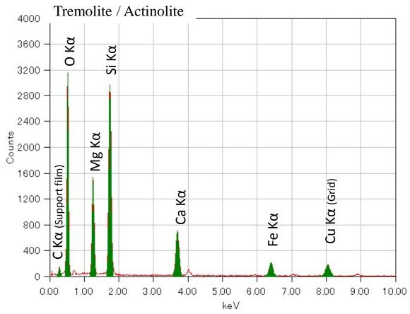
(The spectral peaks of C and Cu are generated from the elements of the support film and the grid.)
