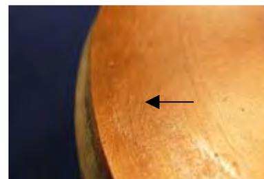
Fig. 1 Organic contamination on metal surface
